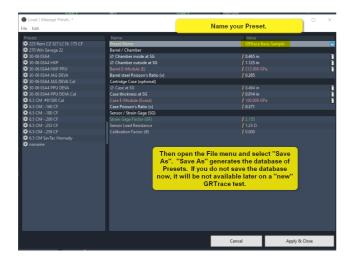
Now that the User has a Barrel Preset, he can start to measure relative pressures in his rifle. There is only the matter of finding out what the other imput fields are for, and where do they appear. First, place GRTrace in Simulator mode as mentioned above. Then fill in the "General File Information's" as required. Take note of where (if they do) appear on the Results screen for "All Traces". Not all show up in the Results screen, some are for User reference while viewing the graphs only.
