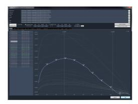
If the law of combustion is used instead of **z(t)**, it can be resolved according to the product of *dynamic vivacity* and form function **phi(z)** (see image/diagram above, Y-axis).
