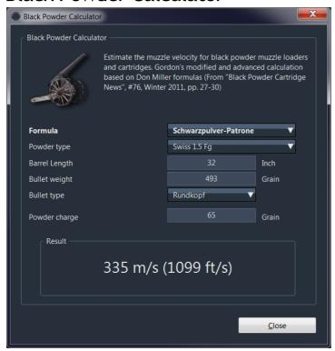
Internal ballistic simulation calculations with black powder are unknown / nonexistent, therefore only rough estimates can be made. The black powder calculator provides the functions for estimating the muzzle velocity.
